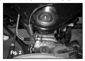
**NOTE:** There are two holes on the top of the spindle where the brake lines mount. On the passenger side, only the rear-most hole is threaded to accept the bolt. For best results, tap the forward-most hole to 6MM x 1.0 thread, using that hole to mount the passenger side brake line and ABS wire.
