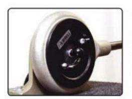
Step Five: Make sure your die number is correct for hose you are crimping. Lift handle to top position opening dies. Place end assemble in dies. Align edge of the collar (at hose) with back face of dies, using over center action push down on handle until assembly releases from crimper. Inspect assembly, be sure to wash & pressure test prior to use.
