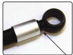
Step Four: Check collar/barb assembly to insure there is no gap (as shown by the arrow). If collar moves freely between hose and end fitting repeat step three.
