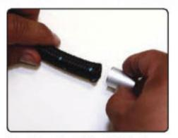
**Step Two:** Install the ProClassic Crimp Collar onto hose.
