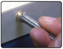
Step Two: Insert the nipple portion of the PowerFlex hose end in a vise. Slip the hose over the nipple using a twisting motion to size the I.D. of the teflon. Separate the wire braid from the O.D. of the Teflon® tube with a small screwdriver. Be careful not to crush the Teflon.
