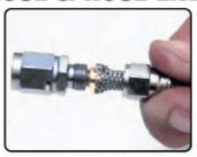
Step Three: Push the olive sleeve around the Teflon® & between the braid. This can be done by pushing the olive sleeve against the side of your workbench or vise. Be sure the Teflon® liner is square to the bottom of the olive. With the nipple in the vise, lube the threads and the nipple portion of the hose end sparingly. Insert the hose over the nipple. Make sure the olive does not pop off tube
