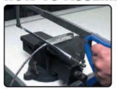
Step One: Wrap the hose tightly with electrical or racers tape. Hold the hose firmly in a vise without crushing and cut through the tape. Make sure you make a straight cut. Remove the tape slowly and deburr the Teflon® edges. Install the socket on the hose and slide it back out of the way.
