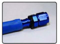
Step Two: Oil inside of hose & barbed end of hose end. Insert barbed end into hose using a twisting action. Put the swivel end at center hex in a vise. Use a twisting motion make bottom of hex even with hose edge, rubber insulator will cover end of hose.
