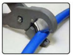
Step One: Cut hose to length using a sharp knife or shears.
