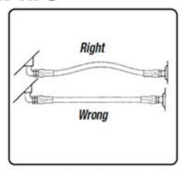
Allow slack in your hose assembly for changes in length that occur under pressure.
