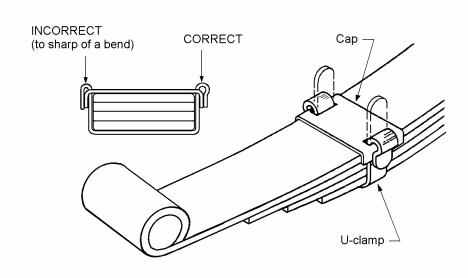
Install a U-clamp (from the bottom) over the leaves and at one of the leaf spring. Place a cap on top of the U-clamp as shown in the illustration. Repeat for other end.
