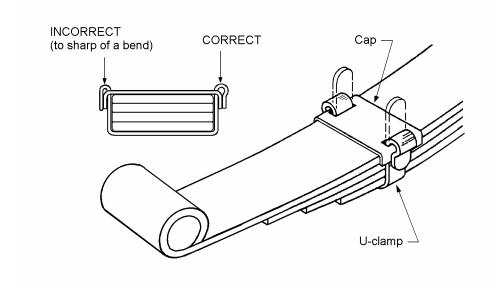
Install a U-clamp (from the bottom) over the leaves and at one of the leaf spring. Place a cap on top of the U-clamp as shown in the illustration. Repeat for other end.
