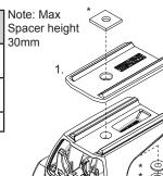
\*Fix the Quick Mount Spacer to the Leg using the hardware in the leg kit. The bolts found in the spacer kit will replace the original in the leg kit.
