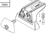
\*Fix the Quick Mount Spacer to the Leg using the hardware in the leg kit. The bolts found in the spacer kit will replace the original in the leg kit.
