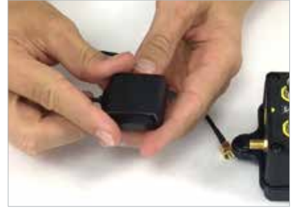
3. The GPS antenna will be mounted horizontal and in view of the open sky.
