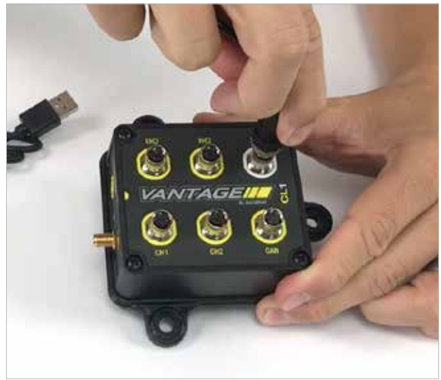
2. Connect Charging Cable Adapter to the PWR port.
