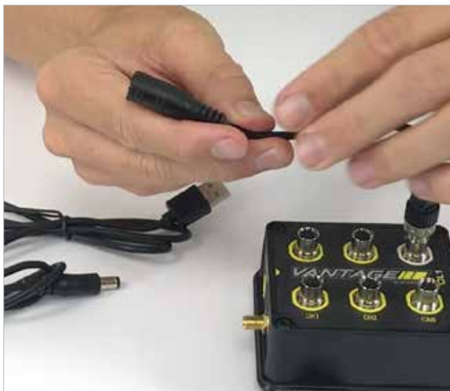
3. If possible, secure the charging port cable to an accessible location via tie wraps, as this will simplify charging of the CL1 Data Box batteries.
