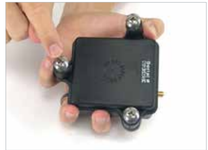
6. The CL1 Data Box can be mounted in any direction, via the three rubber isolation mounting feet.
