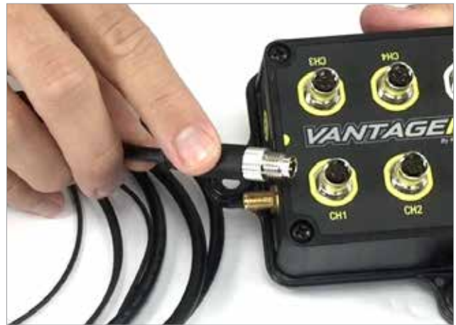
2. Connect the five pin connector to Channel 1 of the CL1 data box.
