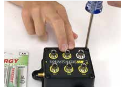
3. Using a small Phillips screwdriver, completely loosen each of the four screws found on each top corner of the CL1 data box.
