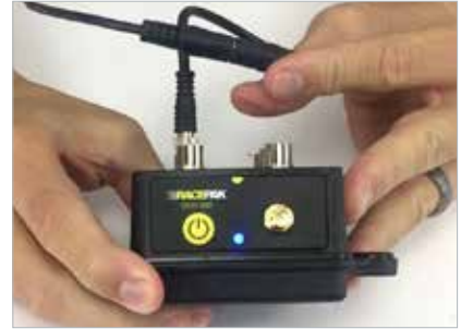
9. Charge the batteries following the Charging the CL1 Data Box Batteries section of this manual.
