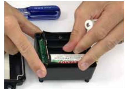
6. Once removed, install each battery, ensuring the battery + and - are oriented as shown on the battery pack case.
