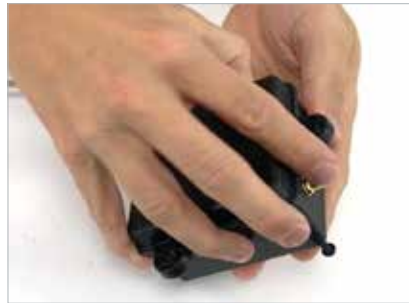
5. Grip the mounting pads and gentle wiggle, while pulling the base from the housing.
