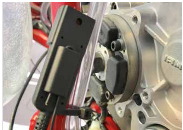
4. Route the opposite end of the cable, containing the molded temperature and engine RPM connector, to a location as close as possible to the motor.
