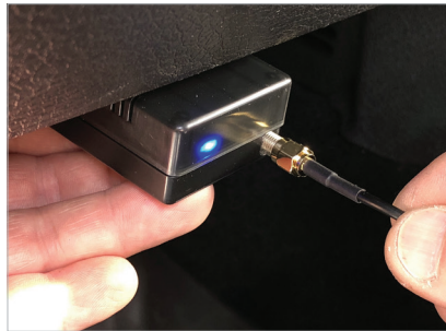
5. Connect the GPS antenna to the GPS connector on the end of the CL2.
