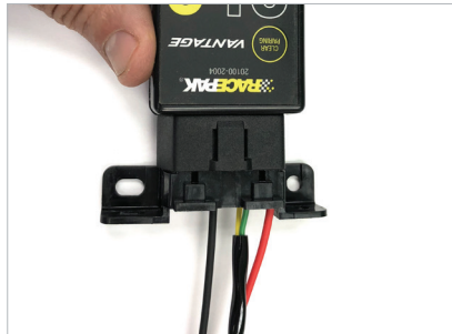
2. Connect the OBD2 to EFI adapter to the CL2.
