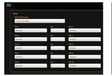
10. Up to 10 ECU channels and desired sample rate (Hz) can now be programmed, one at a time, using the down arrow under each PID input area.
