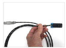
3. Connect the opposite end of the interface cable to the ECU. Connector varies based on ECU.
