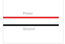
5. Route and connect the oppositeend of the power cable to a switched,12V power source, in the vehicle.Red=Power Black=Ground
