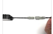
2. Connect the interface cable to the EFI module.
