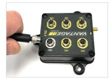
4. Locate the red, three pin power cable included with the Vantage EFI interface module. Connect the three pin connector to the PWR port of the CL1.
