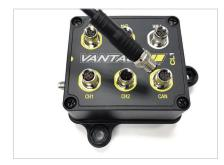
1. Plug the 6 pin EFI cable into the CAN port of the CL1 data box.
