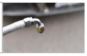
7. Torque the B-Nut on each hose end to the catch can fittings.
