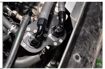
8. If not already, slide a clamp onto the hose and install the smaller factory PCV hose (still in engine bay) to the barbed fitting on the side of the rear most catch can.
