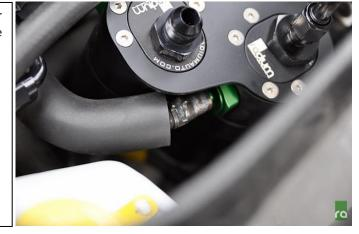
9. The larger PCV hose that was removed in the earlier steps is going to be cut down and used between the port on the throttle body and the larger barbed fitting on the forward most catch can.
