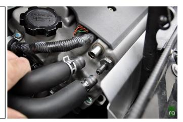
3. Disconnect the larger PCV hose the same way from the port on the throttle body (shown) and remove the hose from the engine bay.
