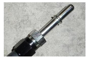
20. Locate the 40" long PTFE hose with 90 degree hose ends on both sides. Secure one of the included adapter fittings (hose barb to -6AN male) to one of the ends of the PTFE hose.
