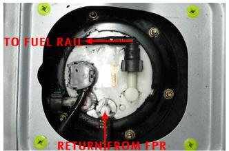
16. Remove the high pressure line from the fuel pump hanger fitting by first squeezing the 2 opposing tabs and then pulling away from the fuel pump hanger fitting.
