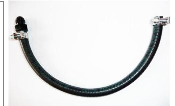
22. Locate the last remaining PTFE hose in the kit which has a 90 degree and a straight hose end that is 41" long.
