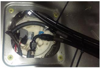
24. With the four hoses routed, test fit the OEM fuel pump access cover. Make a mark on the cover to cut away a section for the hoses and trigger wire to pass through, as shown.
