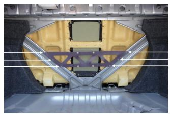
4. Remove the rear seat bench by pulling the 2 levers underneath.
