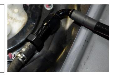
21. Locate the non-permeating  $\frac{1}{4}$ " ID rubber Barricade hose and the other -6AN male to barb adapter fitting in the kit.
