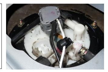
9. Screw in the opposing side of the Posi-Tap connector to lock the white wire in place, as shown.
