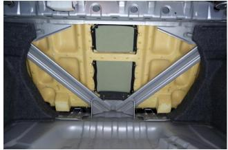
3. Lineup the large flat brace included in the kit to the support beams. Confirm the brace is horizontal using a level.
