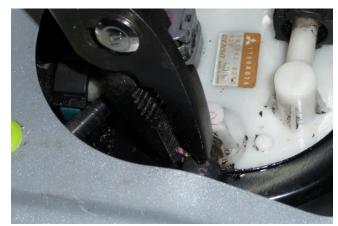
18. Locate the hose in the kit that doesn't have a hose end on one end. Using the included hose clamp, install the female quick disconnect fitting found in the kit, as shown.
