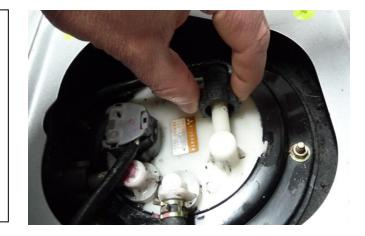
17. Loosen the spring clamp on the return hose with a pair of pliers, as shown.
