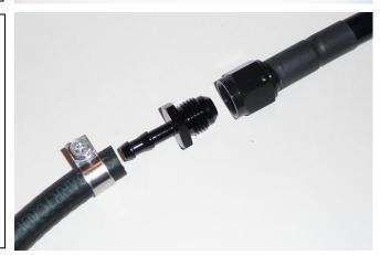
23. If necessary, the FST can be disassembled and the top and bottom caps can be rotated for optimal hose routing. Furthermore, the OEM fuel pump hanger can be rotated clockwise slightly for best hose routing.
