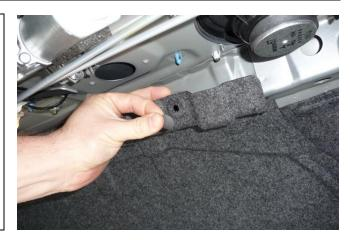
2. Remove the panel attached to the back of the rear seat from the vehicle, as shown.
