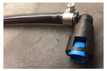
19. Locate one of the 41" long PTFE hoses that has 90 degree hose end and a straight hose end. First, install the quick-connect male adapter into the straight hose end, as shown.
