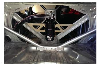
27. Reinstall fuel pump cover, door sills (shown), rear seats, trunk paneling, etc.
