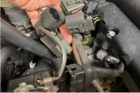
3. Carefully pull the vacuum tubing off the fuel pressure regulator (FPR).
