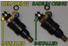
12. If the OEM RB26DETT fuel injectors will be reused, replace the upper O-rings with the six O-rings included in the kit. This will effectively convert the stock 10.45mm (JECS) injectors to 11mm (Denso) fitment.
