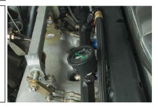
30. After everything is reinstalled, cycle the key a few times (without starting engine). This allows the fuel pump to prime the system. CHECK FOR LEAKS! If no leaks are found, start the engine and check again while the engine is running.
