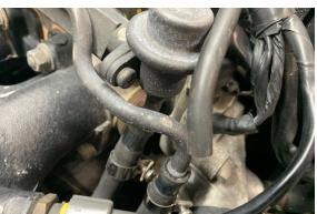
4. Pry the electrical metal locking clips from the six fuel injector connectors.
