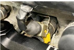
28. If the OEM Nissan plastic injector wiring harness cover will be reused, it might need to be modified if something is installed into the center port or gauge port other than plugs. Shown is the modification required to directly mount a fuel pressure gauge to the rail.
