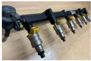
19. For fuel rail mounting, preinstall the 2 bolts, washers, spacers, etc. provided in the kit, as shown.
