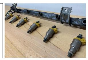
11. The Radium Engineering fuel rail is compatible with 11mm upper injector Orings. This is a very common size for injectors (Denso).
