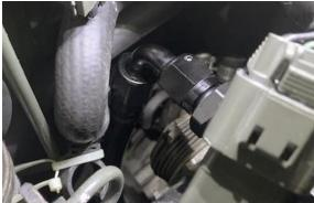
27. Plug in all electrical connections. Reconnect the vacuum hose to the FPR.
