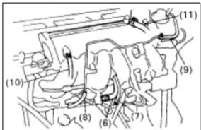
3. Disconnect EGR gas temperature sensor connector.
