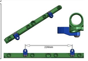
5. To secure the mounting feet to the rails, install the included split lock washer and M5 bolts (as shown).
