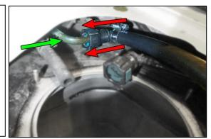
21. Carefully tip the fuel hanger assembly to angle in the fuel level sender float first. Next, readjust vertically and drop the fuel pump hanger down into the tank moving the connectors out of the way one by one.
