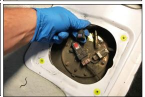
23. To reinstall the OEM fuel feed and return line, follow the steps below. For installing the Radium 20-0376-0X Fuel Hanger Plumbing Kit's feed and return lines, skip these instructions and reference the instructions at the end of this document.
