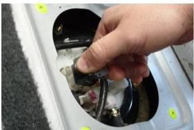
3. To detach the OEM feed line (shown top) and crossover line (shown left), simply squeeze the 2 opposing locking tabs and pull the female fitting away from the male tube. Be careful not to side load the white plastic fittings. Use a rag to clean up any spilled fuel.
