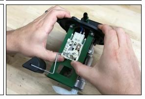
15. Find the OEM rubber gasket that was previously removed from the OEM module. Inspect to make sure there are no rips, tears, cuts, imperfections, etc.
