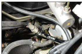
18. As shown, install the provided -6AN male to inverted flare fitting into the OEM "feed" hard line (now converted to a return line).
