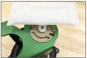
13. Insert the male flat blade terminals from the blue and brown wires into the 2 functioning fuel level sender electrical slots. It does not matter which wire goes into which slot.
