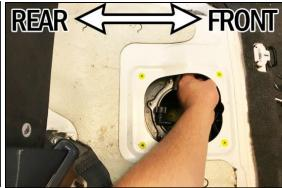
17. Squeeze the 2 blue locking tabs and simultaneously pull the tube off the hard line. Have a rag handy. NOTE: This procedure is much easier without a fuel pump module installed, as shown.
