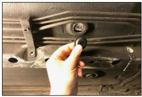
6. Flip the plug around and reinsert until it locks in place, as shown. This will provide additional room for the fuel filter assembly.
