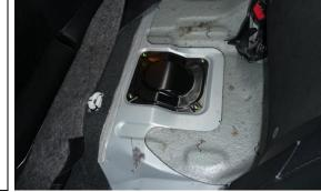
2. To depressurize the fuel system, first squeeze the tab and unplug the gray wiring connector on top of the pump housing (shown). Start the engine and allow it to stall. Remove the key from the ignition. Unscrew the gas tank filler cap temporarily to relieve any residual pressure.
