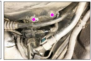
12. Using a pair of pliers or channel locks, reach up and bend the gas tank tab downwards.
