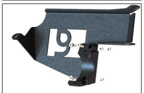
3. Place the fuel filter onto the lower clamp with the green "OUTLET" up against the bracket, as shown. Find the upper portion of the filter clamp and two M5 bolts provided in the kit. Clamp the fuel filter down to the mounting bracket using a 4mm Allen hex wrench.
