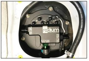
15. Find the -8AN PTFE hose in the kit that has a 120 degree and a straight hose end. Run the PTFE hose through the area mentioned above. Loosely install the 120 degree hose end to the "Pump Out" port (do not tighten yet).
