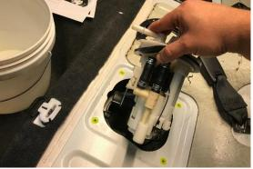
5. The only parts that will be reused from the OEM fuel pump housing is the fuel level sender and large black gasket shown.
