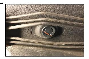
7. Lineup the filter bracket assembly to the open threaded holes. Install the 3 provided button head bolts to the chassis. If necessary, pull and spread the OEM hard lines to permit additional space.
