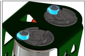
12. This kit was designed to be used with a specific filter sock (RADIUM P/N: 14-0143). Large fuel pump filter socks may NOT fit properly. Press the filter sock(s) onto each pump inlet and secure with the star washer (shown).
