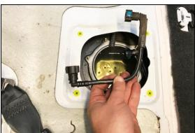
18. Using a utility knife blade, carefully cut a slit into the barbed end of the SAE quick connect fitting and remove the hard plastic tube, as shown.
