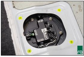
16. From underneath the vehicle, be sure the -8AN PTFE hose is free of obstruction, sharp edges, suspension components, hot exhaust, etc. Connect the -8AN straight hose end to the black fuel filter "INLET" fitting (do not tighten yet).
