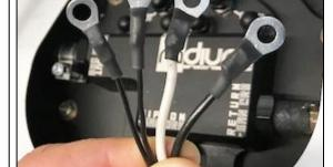
27. Attach the ring terminal with the large gauge (AWG) black wire to the ground "GND" pump-1 terminal.
