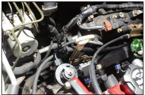
20. Find the last -8AN PTFE hose end in the kit. Install the 45 degree hose end to the fuel rail. Radium 20-0029 Fuel Pressure Gauge and 14-0148-08 Inline Adapter Fitting is shown. Route the hose down towards the hard lines staying clear of any hot or moving parts.
