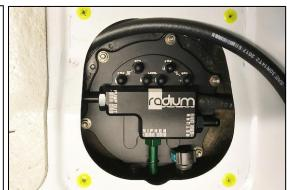
22. The OEM crossover will be slightly too long to connect as-is. A trick is to remove the RH access cover on the passive side of the gas tank using a Phillips head screwdriver. Squeeze the 2 blue locking tabs on the crossover fitting and simultaneously pull off, as shown. Have a rag handy.
