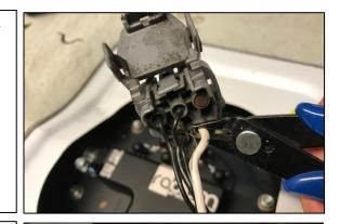
26. Cut two ½" pieces of the small diameter shrink tube. Insert onto each sensor wire (two small gauge wires). Next, crimp on a small gauge (AWG) ring terminal to each wire. Slide the shrink tube over the crimped section of the ring terminal and shrink into place with a heat gun.
