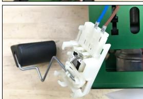
14. Next, insert the fuel level sender unit through the fuel pump hanger bracket slots towards the bottom. Carefully slide the fuel level sender upwards until the white plastic tabs lock onto the Radium fuel hanger bracket.
