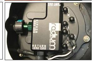
$28.\ \underline{\textbf{Optional:}}\ \textbf{Radium Engineering recommends upgrading to high current wiring.}$
