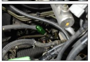
19. Find the -6AN PTFE hose in the kit. Install the 45 degree hose end to the -6AN to inverted flare fitting. Install the 90 degree hose end to a -6AN return fitting on the FPR (not included).
