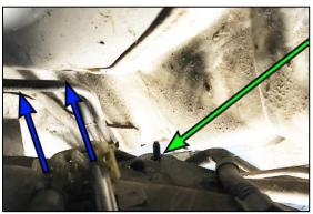
11. From underneath the car, find the two ABS electrical connector hold down clips. Dislodge the plastic clips so there are simply two holes, shown in purple.
