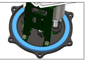
16. If the OEM fuel lines will be reconnected or if the Radium 20-0276-0X Fuel Hanger Plumbing Kit will be installed, there is a short OEM fuel tube that will need to be removed.
