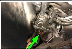
9. To drop the fuel tank down a few inches and allow extra working room, remove the 4 nuts shown using a 14mm socket wrench.
