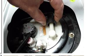
4. Before removing the OEM fuel pump housing, place an empty bucket nearby. There will be residual fuel in the gas tank. Slowly lift the canister straight up then tilt the fuel pump housing towards the RH side to clear the level sender float, as shown.
