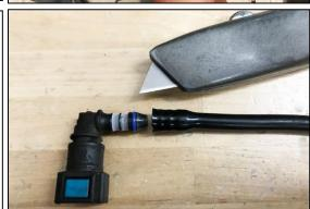
19. Insert this OEM SAE quick connect barb into the included short rubber fuel hose. Secure with the provided EFI clamp.
