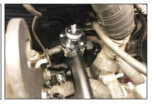
68. Secure the return line near the fuel filter using one of the provided cable zip ties, as shown.
