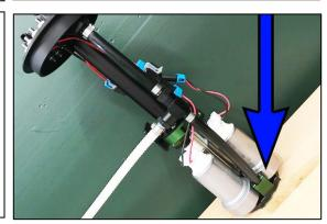
22. If there are plans to have ALL pumps running at the same time during low engine loads (low demand), excessive backpressure could potentially be present in the return. This will make low static fuel pressure hard to obtain. If this is true, remove the Radium venturi system and all 3 corresponding tubes. Follow the instructions below to revert back to mimic the OEM return.
