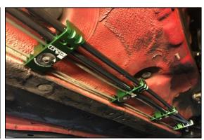
73. After tightening all related fittings, secure the fuel filter clamp using a 4mm Allen hex wrench. Notice how the filter is slide upwards inside the clamp to add ground clearance.
