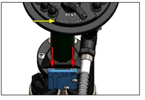
24. Find the 3 sensor wires hanging from the fuel hat. Match each wire color and push each terminal into the OEM 3-pin connector (see yellow arrow pictured).
