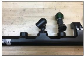
81. Apply a small amount of PTFE paste to the pressure gauge threads and install into the elbow fitting, as shown. Use a 7/16'' wrench to tighten the gauge and a second wrench to hold the elbow fitting.
