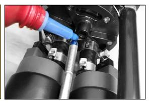
18. If installing 1 or 2 fuel pumps, screw in the bolt (shown red) with a 10mm socket wrench just enough before the filter assembly becomes crooked. Do NOT tighten! Use the included filter support bracket (shown blue) and the screws (shown yellow) to keep the assembly straight.
