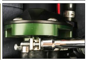
17. To install the top portion of the lower fuel pump filter screen, the fuel pumps may need to be clocked to mate into the holes to line up (2 holes per pump). Once properly positioned, press towards the pump(s) until each is fully seated (see the following step's picture).
