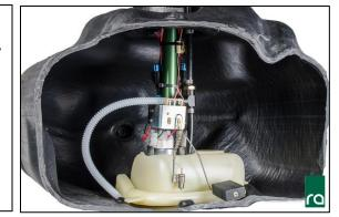
30. To reinstall the OEM black hold-down ring, rotate clockwise and tighten. NOTE: The top 3 fittings can freely swivel for additional space.
