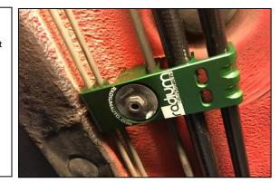
70. Just in front of the LH half shaft, the OEM hard lines make tight bends. For optimal fuel flow, the replacement fuel lines will bypass this potential restriction.
