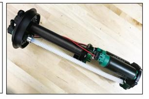
23. If not installed already, secure the Radium fuel sensor mount to the rear-most area of the triple pump block. Two of the bolts from the triple pump block will first need to be removed. Referencing the picture at the right, note the "REAR" engraving on the fuel top hat and the 2 bolts on the "rear" of the triple pump block.
