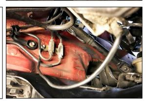
63. NOTE: for this plumbing kit to connect properly, the fuel rail (not included) must have an 8AN ORB threaded front port. Radium Engineering recommends, 2JZ-GTE Fuel Rail P/N: 20-0215. Install the included 8AN ORB to 10AN male fitting to the front port of the fuel rail.
