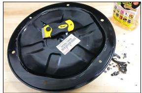
43. Find the adhesive foam included in the kit. Peel the backing off and apply on the flat areas around the cover on the inside of the 6 mounting holes (shown in blue). Cut to length.
