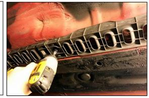
$51. \ \mbox{Pry}$  the locking tabs to release the plastic hard line covers.
