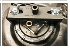
4. Before removing the OEM unit, place an empty bucket nearby as there will be residual fuel in the gas tank. Slowly lift the assembly straight up.
