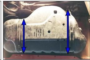
66. The new fuel lines will be routed in the same manner as the OEM fuel lines. From the trunk, first slide the long 8AN feed line down the front LH side opening.
