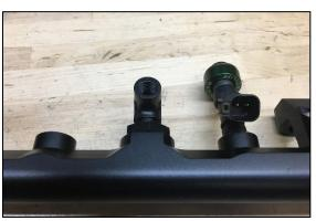
79. Using the same PTFE paste and tightening procedure as the first 1/8NPT elbow, install the second elbow into the outlet of the first elbow, as shown.
