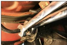
46. Using a 10mm socket wrench, remove the ground wire ring terminal bolt. NOTE: This could be found on any one of the 3 bolts shown.
