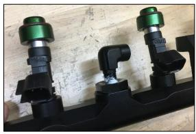
78. NPT threaded fittings should first be tightened finger tight. Then, using a wrench, add another 1.5 to 3 turns until fully tight and pointing straight up (same direction as the injector electrical connections).
