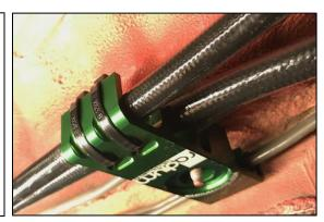
72. NOTE: the rearmost retainer will not require zip ties as the retainer touches the floorboard.
