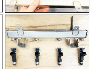
6. The 4 OEM fuel injector locking clips will be reused.
