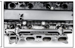
10. As a test, push the fuel injectors downward until they bottom out. Now inspect the injectors' upper O-rings and confirm they are still inserted into the fuel rail injector bores. Do not pressurize the fuel system until the proper height is achieved.
