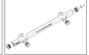
8. Lubricate each fuel injector's top O-rings with engine oil. Fully insert the fuel injectors into the Radium fuel rail injector ports. If reusing OEM or compatible fuel injectors, slide the OEM injector clips on locking them to the fuel rail.
