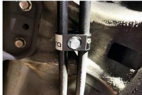
7. Route the 2 fuel hoses up in front of the fuel tank so they can be accessed from the LH access panel inside the vehicle.
