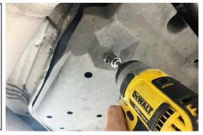
3. Temporarily remove the protective shield from the vehicle.
