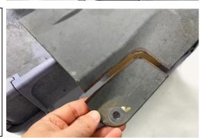
8. There are seven bolts along the outer RH side underneath the vehicle. For this kit, remove the five middle bolts using a 10mm socket. NOTE: The front and rear bolts are too far away to be useable.
