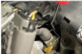
5. Be careful not to lose the metal fuel injector clips in the engine bay.
