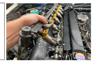
10. Remove the fuel rail from the vehicle. It will contain fuel.
