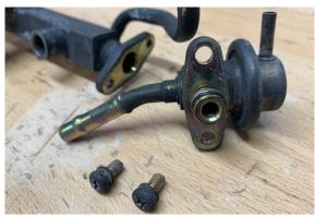
17. If reusing the OEM FPR, first lubricate the O-ring found on the black threaded portion of the adapter. Next, tighten to the front port of the fuel rail.
