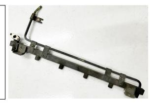
11. Reference the 2 OEM fuel rail pictures. Note that there are a couple different variations for the RB20DET engine.
