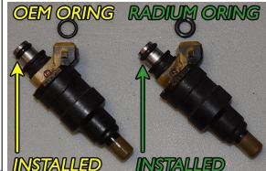
13. If the OEM RB26DETT fuel injectors will be reused, replace the upper O-rings with the 6 O-rings included in the kit. This will effectively convert the stock 10.45mm (JECS) injectors to 11mm (Denso) fitment.
