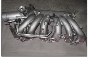
4. After the engine has cooled, place shop towels down under the fuel inlet pipe. Slowly loosen the banjo bolt and catch any gasoline that drips out.
