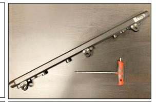
6. Using the OEM fuel rail spacers, position the fuel rail assembly onto the intake manifold. Install the OEM M8 bolts and torque to 15ftlbs (21Nm) using a 12mm socket wrench.
