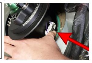
45. Using the tool and socket wrench from earlier, reinstall the lock ring, as shown.
