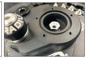
51. A sensor, gauge, etc. (not included) is required to calibrate fuel pressure. A 3/8" wrench and a 3/32" Allen wrench is required to make fuel pressure adjustments.
