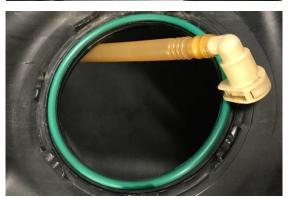
43. Push the OEM crossover line over the Radium SAE quick connector until it "clicks" in place.
