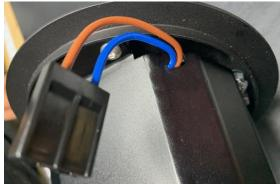
42. Secure the fuel level sensor using the collector box Allen screws. Plug in the electrical fuel level sensor connectors.
