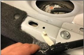
5. It is recommended to clean the top of the fuel pump housing and the surrounding area. This will prevent loose dirt from falling into the gas tank.
