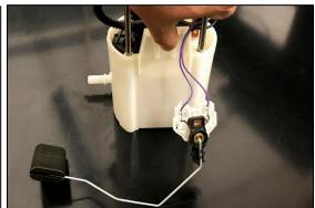
14. Strip the ends of the wires. Crimp the included flat male wire terminals to each wire using a tool such as Molex 63811-1000 hand crimper.
