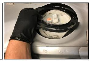
10. Before removing the OEM fuel pump housing, place an empty bucket nearby. There will be residual fuel in the gas tank. Slowly lift the canister straight up.
