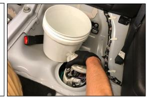
11. Next, tilt and twist the assembly to clear the fuel float arm. Pay close attention not to bend or damage the fuel float arm. Once the float clears, the crossover hose will be visible. Squeeze the thumb tab and pull away to release the crossover hose, as shown.
