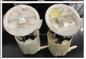
13. Remove the fuel level sensor from the OEM fuel hanger by gently pulling the thumb tab outwards. Do NOT use excessive force! Simultaneously press downwards to release the sender. Depress the 2-pin wiring thumb tab from underneath the top plate and unplug the connector.
