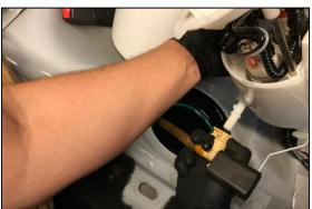
12. For S197 Ford Shelby GT500 (pump unit shown at left), a post-pump filter is already externally mounted underneath the car so a low micron aftermarket fuel filter is NOT necessary.
