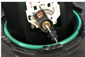
44. It is normal to have a slight interference with the fuel level sensor. When sliding the fuel level sensor past the tank opening, gently push the sensor inward, as shown.
