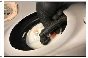
6. Press the thumb button and pull the female fitting away from the male connection. Use a rag to clean up any spilled fuel.
