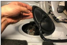
3. On top of the fuel pump housing, slide the electrical connector's red locking tab to the side. NOTE: Because the Shelby GT500 uses 2 fuel pumps, the 2-row connector (shown) is slightly different than other Ford models. All related steps still apply.
