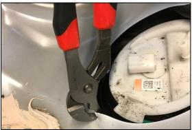
9. Remove the OEM fuel tank lock ring. Note that the OEM Ford pump module is spring-loaded and will pop up as soon as the lock ring is disengaged.
