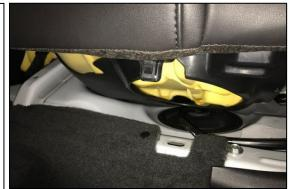
2. Unseat the rubber gasket by pulling up around the perimeter of the large sheet metal hole.
