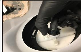
7. To release the OEM hold-down metal ring it is recommended to us a special fuel tank lock ring tool such as OEM Tools, P/N: 24398 (shown).
