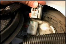
4. To gain maximum access to the fuel pump area, dislodge the wiring strain relief connection shown. Move the connector and rubber cover out of the way.
