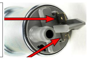
16. If the Walbro F90000274 E85, Walbro GSS342 255LPH, AEM 50-1000 Gas, AEM 50-1200 E85, etc. was purchased, it's required to crimp the included male spade connectors to the included flying lead harness.
