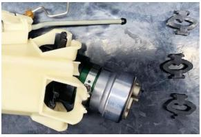
20. From the outside, push the 3 rubber grommets inwards to secure the fuel pump to the OEM unit, as shown.
