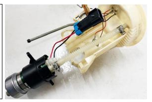
19. Push the fuel pump up into the OEM unit WITHOUT the rubber grommets installed.
