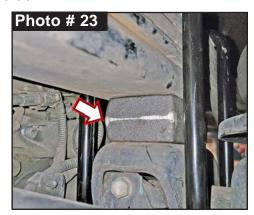
\wrench. Torque u-bolts evenly using an 'X' crisscross tightening sequence. Torque 125 ft-lbs.
