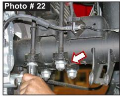
6. While checking for appropriate slack in ABS lines, brake lines, rear emergency brake cables, & etc. Lower axle away from leaf springs to allow clearance for block.
