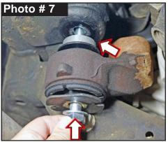
Tighten to All Four (4) Differential Mounts. Torque 120 ft-lbs. Remove jack from differential.
