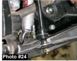
26. Install the new Skyjacker anti torque link by installing the bushing in the eye of the assembly. Attach the eye at the new Skyjacker crossmember using the 1/2" hardware supplied. Adjust out & attach the rod end to the lower ear on the differential using the inserts & 9/16" hardware supplied. Once installed, tighten the jam nut. (See Photo # 25)
