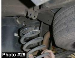
31. Disconnect the OEM upper & lower control arms from frame rail. Only remove one side at a time so that the axle does not move. Install the new Skyjacker upper/lower arm relocation bracket.
