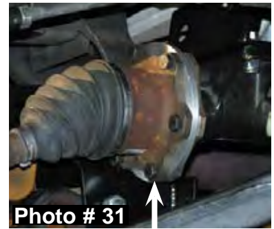
Photo # 31 Passenger side shown with one 15/16" C.V. spacer.
