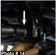
30. Tighten the supplied jam nut of the new Skyjacker adjustable front track bar using a 1 1/8" wrench.
