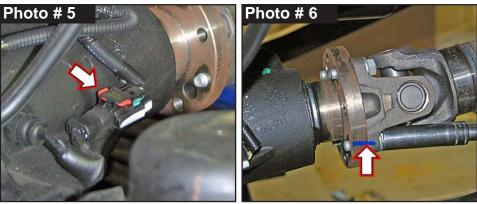
drive shaft does not bind when installing taller springs. Mark the location of OEM front drive shaft\flange at axle & disconnect using a 15mm socket\wrench. (See Photo # 6)
