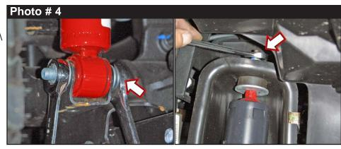
Disconnect OEM front brake line bracket using a 10mm socket\wrench.
