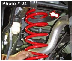
isolator is properly aligned with coil & upper coil spring mount. (See Photo # 24) Raise rear axle to load Skyjacker rear coil springs.
