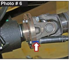
drive shaft to ensure the drive shaft does not bind when installing taller springs. Mark the location of OEM front drive shaft\flange at axle & disconnect using a 15mm socket\wrench. (See Photo # 6)
