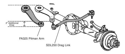
NOTE: This diagram is shown for models equipped with Dana 60 front axles. On Dana 44 axles, the #SDL250 drag link installs from the bottom of steering arm on axle housing instead of the top as shown in the diagram at left.
