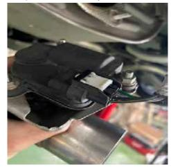
Disconnect wire harness from electronic actuators, Using a suitable exhaust pipe cutting tool, cut completely through the stock exhaust in the two (2) locations shown below. Unhook each exhaust hanger from the sub frame and remove each muffler assembly by sliding the inlets down and forward to extract the rear exhaust hangers from their mounts.
