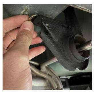
9. Remove the two (2) IRS sub frame mounted exhaust hangers from the stock exhaust system and slide them onto each side of the ROUSH exhaust.
