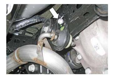
4. Remove electronic actuator, flange nuts, spring, and backing plate from mufflers to be removed. Set aside to be used later for install on Roush active valve assemblies.
