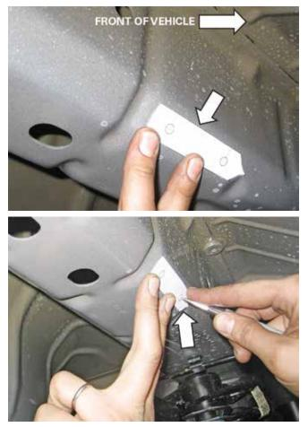
Drill all four (4) pilot holes that were marked in the previous step with a 1/8" drill bit followed by a 17/32" drill bit.
