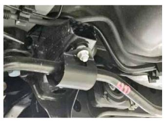
2. Locate the template onto the rear chassis sub frame as shown in the pictures below and mark the drill holes with a center punch. Use the same template to mark the holes on both the RH and LH sides of the vehicle.
