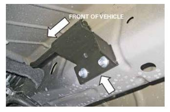
6. Remove both LH and RH exhaust hangers from vehicle with a 13 mm socket. Prepare to cut both hangers with cut off tool of choice (example: cut off wheel).
