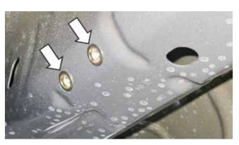
Install the two (2) supplied exhaust hangers (P/N: 1315-5A261 and 1315-5G298) and four (4) bolts (P/N: W500224) as shown below. Torque to 18 lb-ft (25 Nm).
