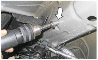
4. Deburr the drilled holes and apply automotive clear coat. Install four (4) rivet nuts (P/N: 95105A191) using the supplied bolt and nut from the rivet nut installation kit (P/N: R1315-5231HWK). Insert the nut onto the bolt and thread the bolt into the rivet nut. Hold the nut with a 17 mm wrench and tighten the bolt nut with a 10 mm socket until the rivet nut is fully seated.
