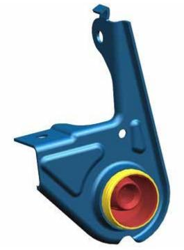
Locate (2) washers - 3/8" X .406" ID X 0.812" OD (11101304). Place them in between the modified bracket and the frame of the vehicle. Reinstall the modified exhaust hangers with the takeoff flange bolts. Torque to 25 Nm. (18lb.ft).
