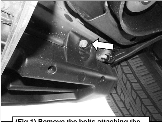
(Fig 1) Remove the bolts attaching the factory running board to the floor panel
