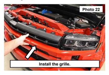
22. Press the grill into the vehicle seating the 8 clips in the center and the 4 clips around the head light on each side of the vehicle.
