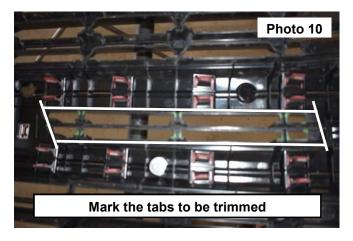
10. Using a body saw trim the bars marked and remove. Use a file or a sander to smooth the edges of the grille were the center bars were removed. **See Photos 11 and 12.**
