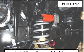
Install the coil spring & isolator.
