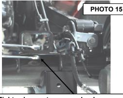
Tighten bump stop spacer hardware.
