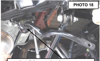
Install the sway bar drop spacer.
