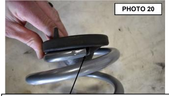
Make sure the coil is properly seated in the isolator.
