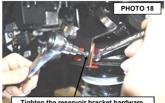
Tighten the reservoir bracket hardware.
