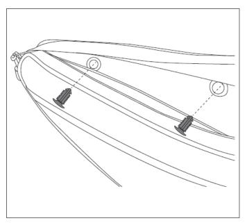
5. Open the zipper inside the bag. Align the holes in the door bag to the drilled holes on the lower door.
