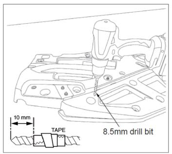
4. Before drilling, wrap a piece of tape around the drill bit 10 mm from the tip to serve as a drill stop.
