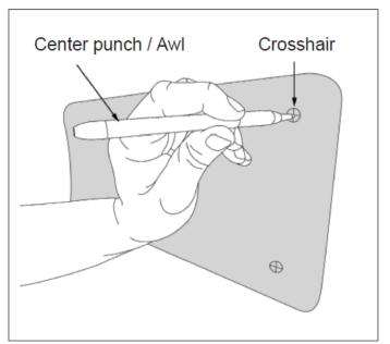
3. Using a center punch or awl, mark center of each crosshair on the drilling template, then remove it. Marked points remain on the lower door.
