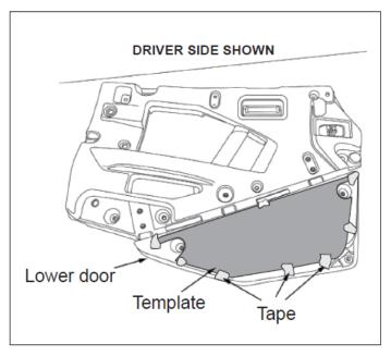
2. Line up the drilling template to the assembled lower door, then tape it in place.
