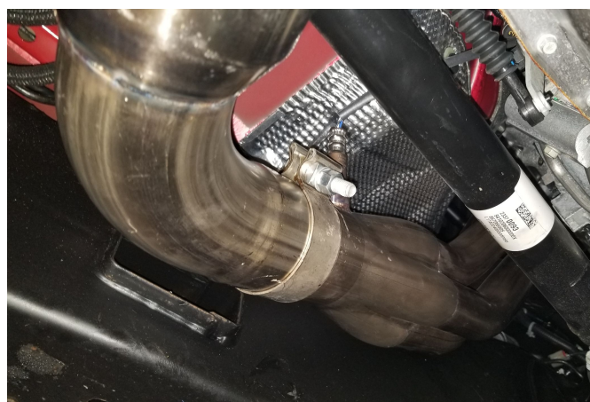
Detail 18: Driver side header - lead pipe connection.
