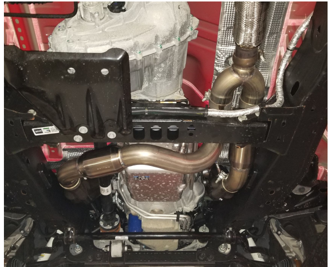
Detail 16: Headers and leads installed
