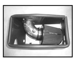
Step 7 Install the supplied air filter and clamp and tighten the clamp that secures the air filter.
