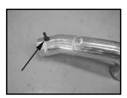
Step 7 Install the supplied grommet into the intake tube and then install IAT sensor into the grommet.
