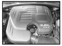
Step 2 Remove the engine cover.
