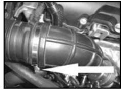
Step 3 Loosen the hose clamp securing stock intake tube to box.
