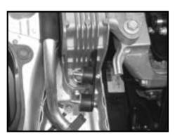
Step 7 Install the heatshield mounting bracket onto the motor mount using the factory bolt removed in step #5.
