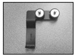
Step 6 Install rubber mounts onto heat shield mounting bracket as shown.
