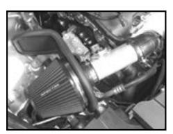
Step 14 Install the filter and securely fasten to the velocity stack adapter with provided hose clamp.
