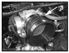
Step 7 Install the coupler on the throttle body and secure the coupler in place. Install a second clamp but do not tighten at this time.
