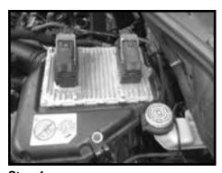
Step 4 Remove the three bolts securing the ECU and the ECU ground to the air box lid and the flip the ECU over and lay it on the valve cover. Note: It is not necessary to disconnect the ECU electrical connections.
