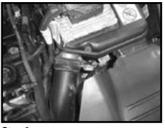
Step 3 Disconnect the inlet air temperature sensor connector. Loosen the hose clamp at the air box. Then disconnect the crank case vent hose from the valve cover.
