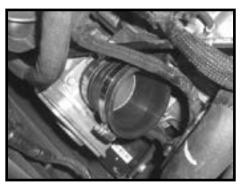
Step 13 Install the provided coupler onto the throttle body and secure with the provided hose clamp.
