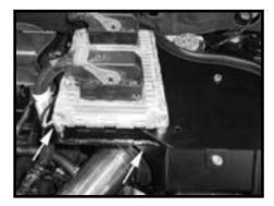
Step 21 Install the ECU support bracket to the ECU making sure to install the ground strap. Then using two bolts secure the ECU mount bracket to the heat shield.
