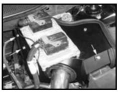
Step 20 Secure the heat shield lid to the heat shield using three provided bolts.
