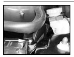
Step 22 Secure the heat shield lid to the inner fender with the provided hardware.
