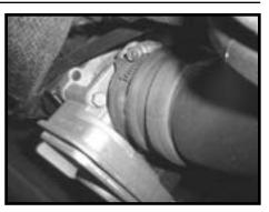
Step 7 Loosen the hose clamp securing the stock intake tube to the throttle body and then remove the intake tube from the vehicle.
