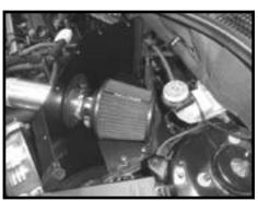
Step 17 Install the air filter onto the intake tube and secure with the provided hose clamp.
