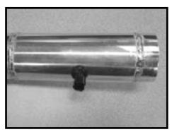
Step 15 Install the provided grommet into the Spectre intake tube then install the inlet air temperature sensor into the grommet.
