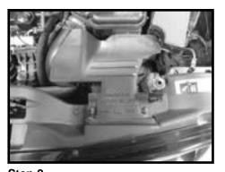
Step 2 Release the two lock tabs securing the fresh air intake scoop and then remove the fresh air intake scoop from the vehicle.
