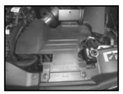
Step 18 Install the fresh air intake scoop into the heat shield and the secure it to the core support with factory clips.
