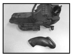
Step 15 Disconnect the fresh air scoop from the stock air box.
