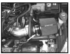
Step 21 Install the air filter and secure with the provided hose clamp.
