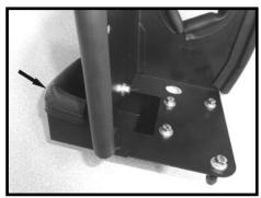
Step 12 Install the 7" section of edge trim onto the fresh air intake scoop as shown. Attach the fresh air intake scoop onto the heat shield using the provided hardware.
