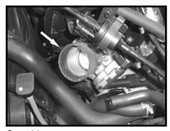
Step 14 Install the provided coupler onto the throttle body and secure with provided hose clamp.
