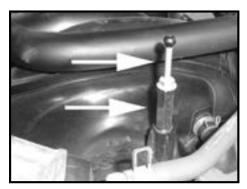
Step 14B (Trucks with 5.7L Engines) Install the provided stud extension onto the stud as shown, then install the stock mounting stud into the extension. Install engine cover.
