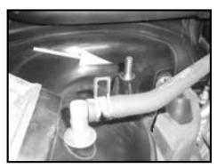
Step 14A (Trucks with 5.7L Engines) Install the provided stud into the mounting stud location as shown.
