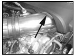
Step 13 (Trucks with 4.6L Engines) Install the factory engine cover. You may have to trim the engine cover slightly so that it does not interfere with the new intake tube.
