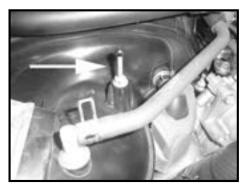
Step 14 (Trucks with 5.7L Engines) Remove the front engine cover mounting stud from the intake manifold.
