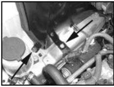
Step 8 Step 8A Step 8B Install heatshield into truck as shown. Some vehicles may have alarm system horn in place on the fender well. Secure the heatshield using the supplied hardware as shown in Step 8A. Then using the factory hardware, secure the heatshield as shown in picture Step 8B. The horn may have to be relocated in order to bolt in the heat shield.
