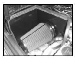
Step 12 Install air filter onto velocity stack. Tighten clamp fully.
