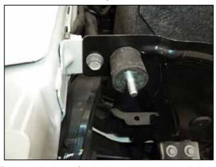
5. Remove the inner fender brace bolt and install the provided rubber mounted stud.
