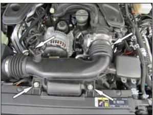
3. Disconnect the crank case vent line from the factory intake tube. Remove the bolts that secure the factory tube to the fan shroud, then loosen hose clamp at throttle body.
