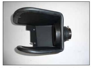
9. Install the filter adapter and coupler onto the heat shield using the provided hardware.
