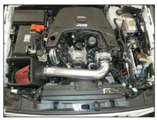
13. Make sure that all clamps and hardware are fully tightened. Reconnect the battery cable, start the vehicle and let it warm up. Shut off and inspect the installation once more for any loose clamps, wires, or hardware. Test drive & enjoy! Your installation is now complete. Periodically check all clamps and brackets.
