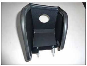
8. Install the provided edge trim onto the heat shield as shown. Install the two provided mounting studs onto the heat shield using the provided hardware.
