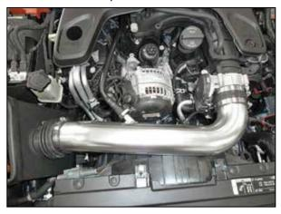
11. Install the intake tube into the coupler at the heat shield and then into the coupler at the throttle body, adjust the tube for best fit and then secure with the provided hose clamps. Connect the crank case vent to the fitting on the intake tube and reconnect the inlet air temperature sensor electrical connection.
