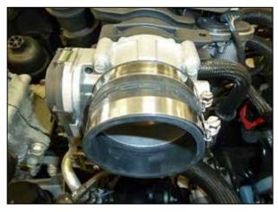
6. Install the provided coupler onto the throttle body and secure with the provided hose clamp.
