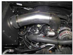
11. Install the SPECTRE<sup>®</sup> intake tube into the flex coupler and then onto the throttle body, adjust the tube for best fit and then secure with the provided hose clamps.
