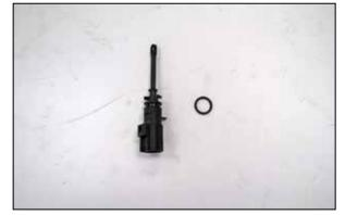
9. Remove the inlet air temperature sensor from the factory intake tube and remove the O-ring from the sensor.
