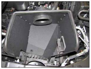
8. Install the heat shield into position as shown.
