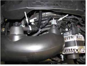
2. Disconnect the inlet air temperature sensor electrical connection and crank case vent line from the factory intake tube.
