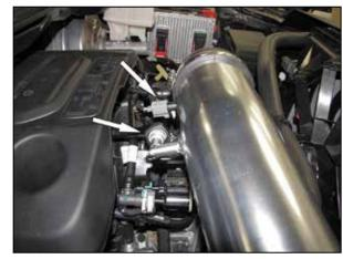
12. Connect the crank case vent line and inlet air temperature sensor electrical connection.
