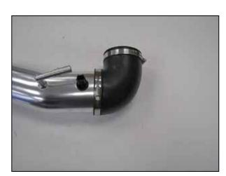
10. Install the inlet air temperature sensor into the SPECTRE<sup>®</sup> intake tube using the provided grommet. Install the 90° coupler onto the SPECTRE<sup>®</sup> intake tube and secure with the provided hose clamp.
