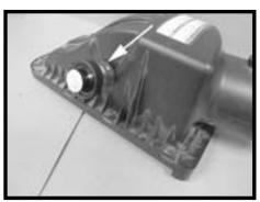
Step 6 Remove the filter minder and grommet from the air box lid.
