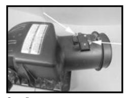
Step 5 Remove the 2 screws securing MAFS from the air box lid. Then remove the sensor from the air box.
