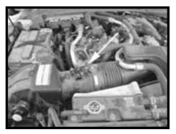
Step 4 Loosen the clamp on the air box lid from the factory intake tube. Remove the air box lid and filter from the vehicle.
