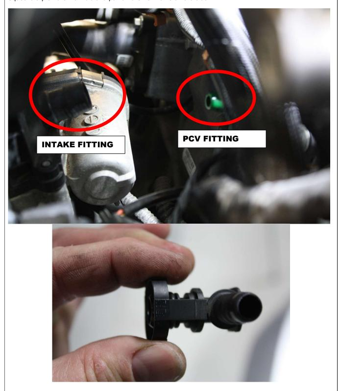
**5** Remove the fitting from the factory hose and install in the 14" ½" hose using the supplied clamp.
