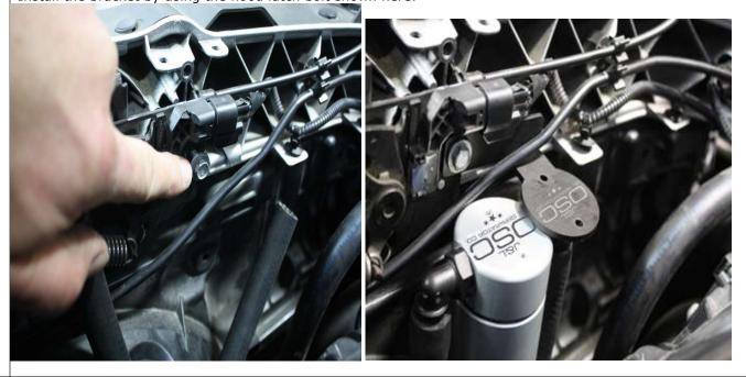
Use OIL on the fittings and insert the hose from the PCV valve (block) to the "C" side and the hose from the manifold to the "O" side of the Separator.
