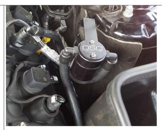
Use supplied screws to mount oil separator to bracket. Run shorter hose to valve cover as shown, route long hose to intake and plug in. The fittings in the end of the hoses will rotate if they need to be adjusted.
