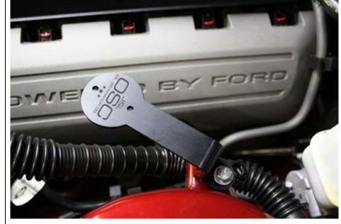
Mount J&L bracket to shock tower tab with supplied nut and bolt
