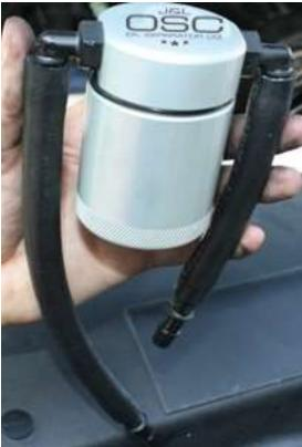
Use the 2 supplied fine thread screws to attach the Oil Separator to the J&L mounting bracket. Mount the Separator so the **J&L LOGO IS LINED UP WITH THE J&L ON THE BRACKET.**
