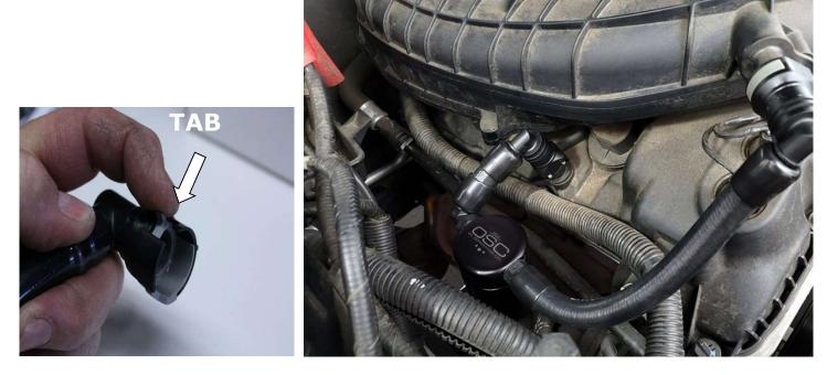
To properly clean the filter in the Oil Separator, spray any degreaser or solvent through it and let it air dry. Clean it every 10,000 miles.
